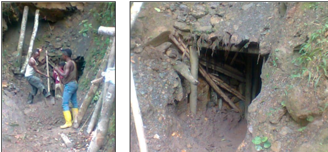
Figure 12. Photograph illustrating the basic structures used to support an artisanal mining site near Bunyakiri - community neighbouring the park. Credit: Blandine Bahati. WCS
